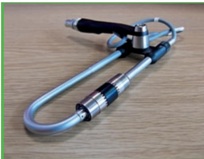
Figure 5. Sound intensity probe
